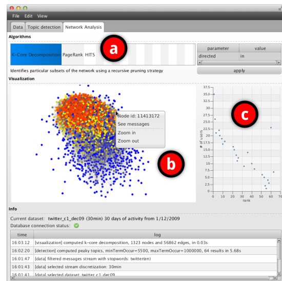
Figure 4: Visualizing a network of authors for a selected topic and time period, colored with k-shells.
